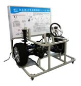
The AT-7004 demonstrator enables learning and getting familiar with the EPS system, the EPS technology, the power control function, the aligning control function, and the high-speed damping control function.
