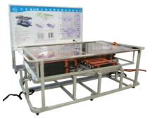
Both the low-voltage control line and the high-voltage power line are original vehicle parts. The high-voltage power line is coated with a protective bellows.
